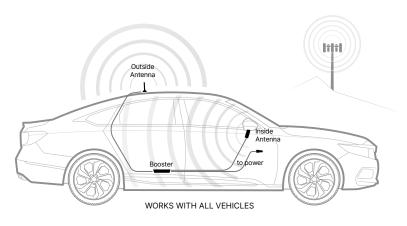
NOTE: For aluminum roofs, an **adhesive disk** is included to mount the outside antenna (do not use if outside antenna will magnetize to the top of your vehicle).
