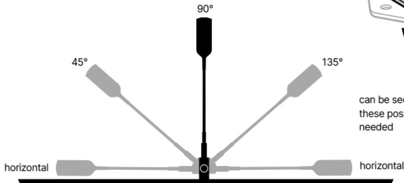
can be secured in these positions if needed
