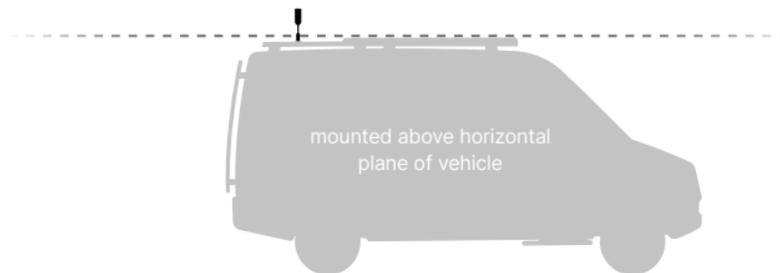
For best performance the outside antenna should be mounted above the horizontal plane of the vehicle and/or above other gear on top of the vehicle.
