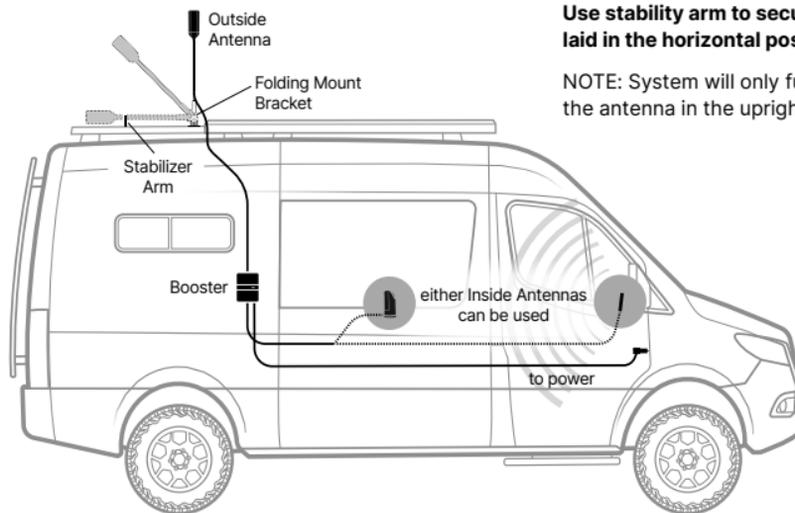
**Use stability arm to secure antenna when laid in the horizontal position.**
