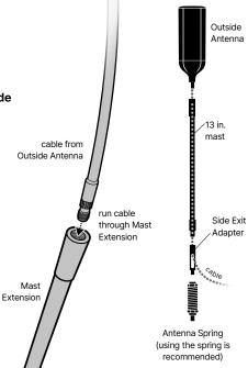
After determining outside antenna assembly is the correct height, **apply the thread locker** precisely to thread points only (not plastic body of antenna). **Screw mast onto antenna**.
