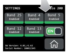
**Bands** can be disabled/enabled by tapping the desired band. Note: disabling a cell band is not recommended. Bands should only be disabled by expert installers.
