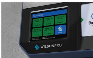
Color touch screen, for easy installation and displaying detailed amplifier status
