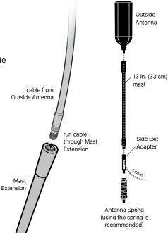
After determining outside antenna assembly is the correct height, **apply the thread locker** precisely to thread points only (not plastic body of antenna). **Screw mast onto antenna**.
